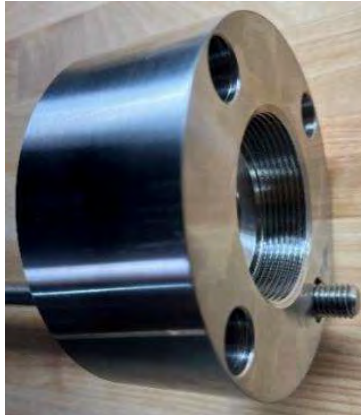
Figure 7. Demonstration of All-thread Rod protruding ¾" from the other side of the Remover Cap.
