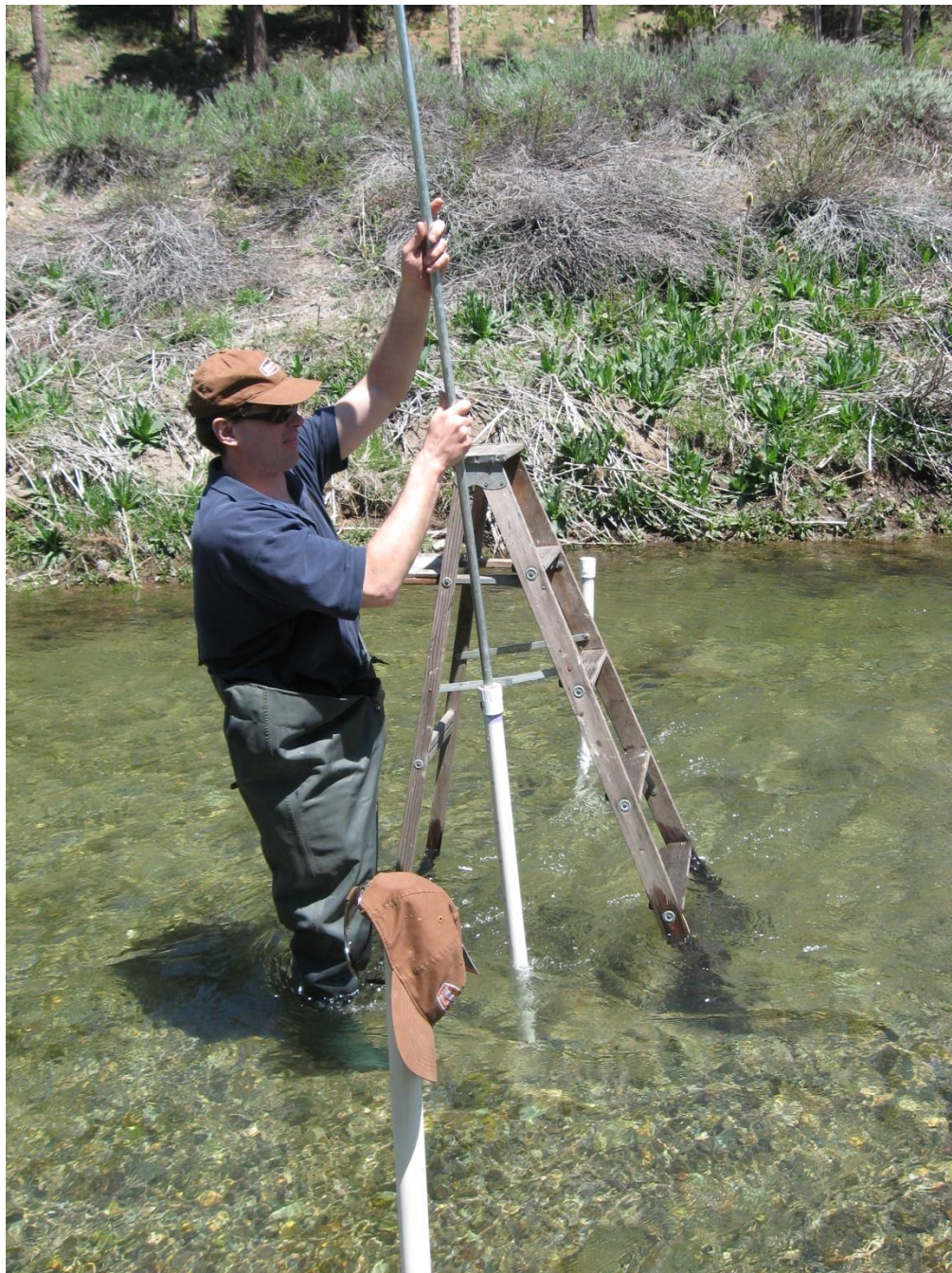
Figure A-1: Temperature Probe Installation
