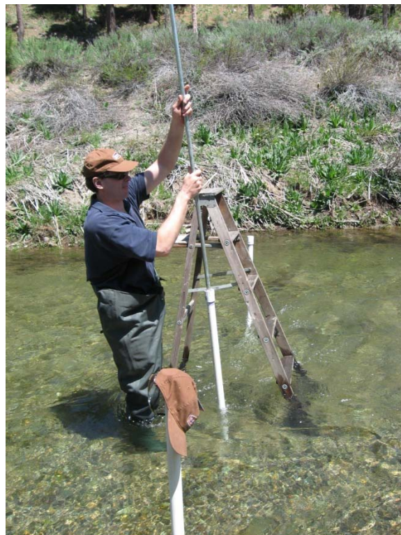
Installing Temperature Probes
