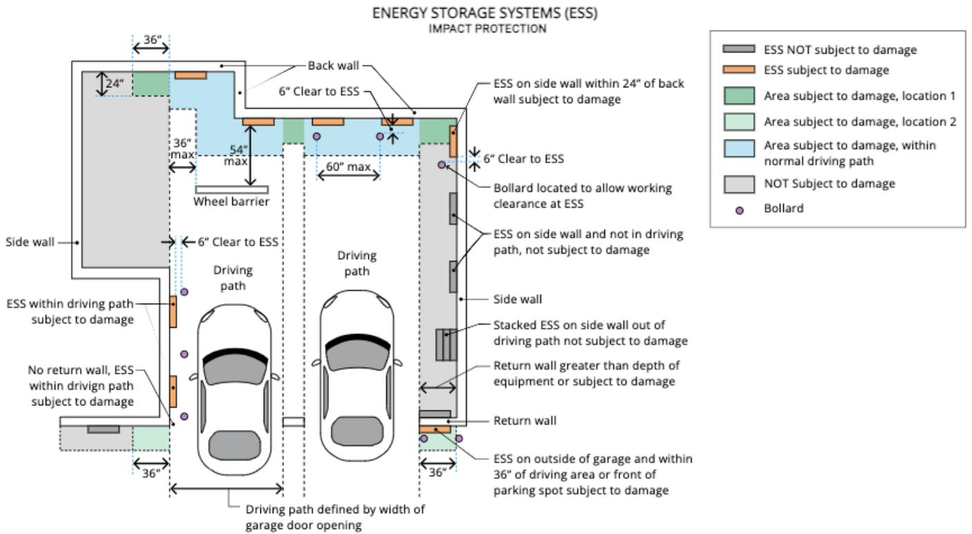
**Figure 3: Energy Storage System Impact Protection (Upcodes CFC 2022 1206.7)**
