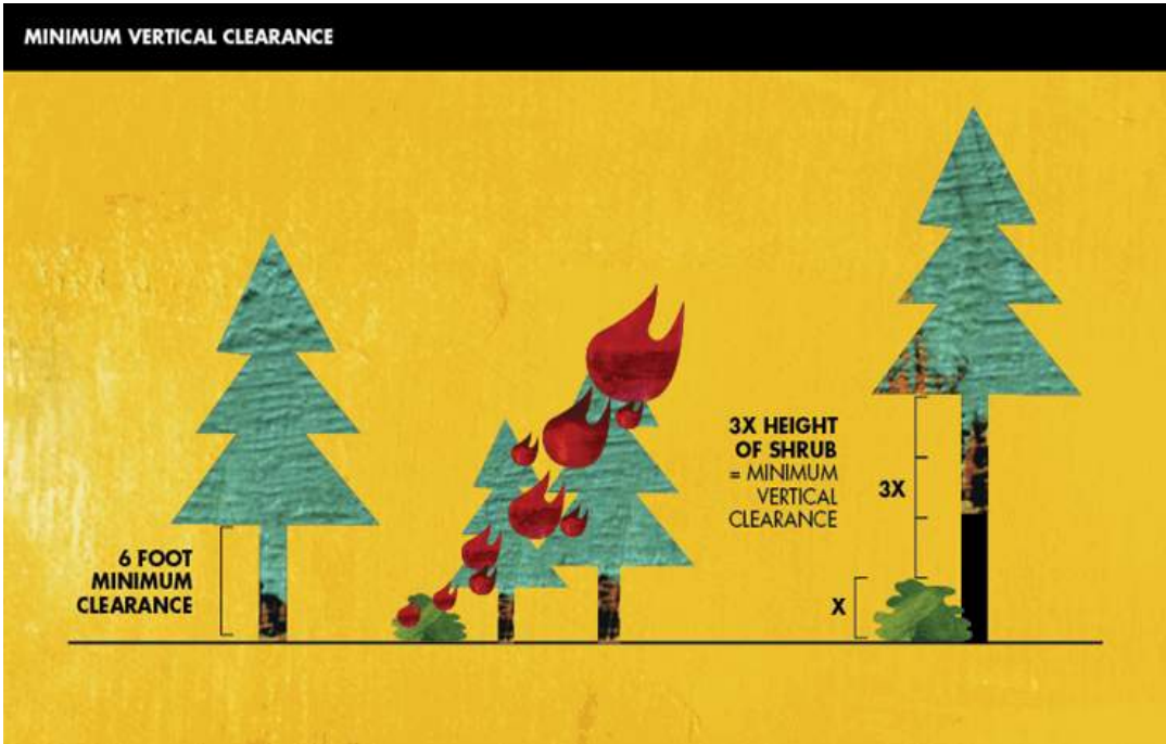
Figure 18: Recommend doubling minimum vertical clearance to 12 feet or 6x height of shrub.
